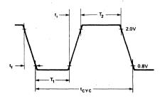
Figure 1. Clock Specification for 8355
